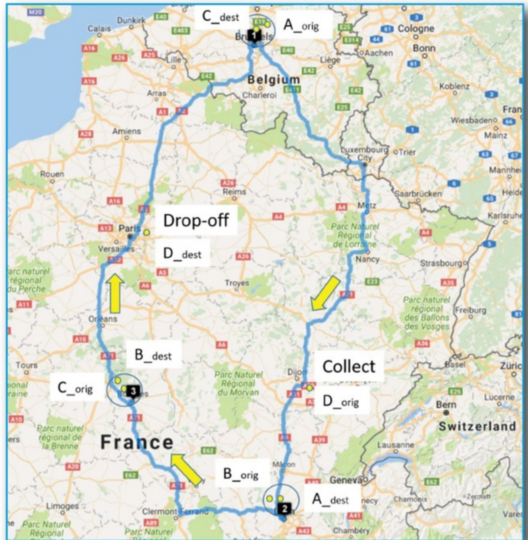
Figure 4: Example of a complex collaboration opportunity. The roundtrip including shipments A, B and C is completed with the collection of shipment D in Dijon as a bundling with shipment A. This shipment D is dropped off near Paris on the route from Bourges back to Brussels (after a bundling with shipment C).
